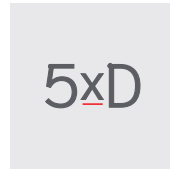
Drilling Depth 5XD
